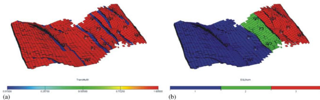
Figure 4. (a) Faults divide model three into three regions and (b) model three has three different regions.
