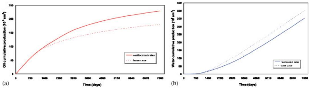
Figure 7. Base case versus reallocated rates case: oil (a) and water cumulative production (b). Model one.
