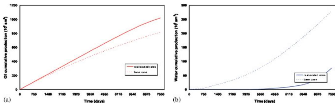
Figure 11. Reallocated rates case versus base case, ECLIPSE check simulation run, oil (a) and water cumulative production (b). Model two.
