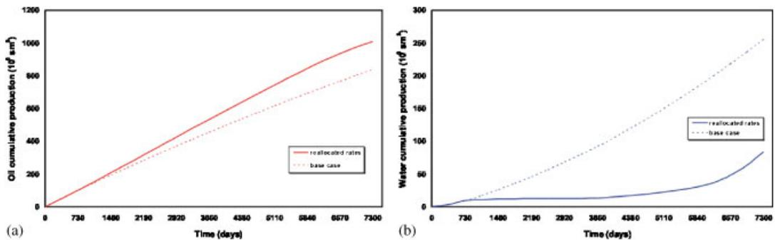
Figure 8. Base case versus reallocated rates case: oil (a) and water cumulative production (b). Model two.
