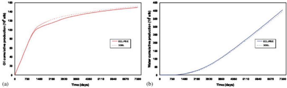
Figure 6. Match ECLIPSE versus 3DSL: oil (a) and water cumulative production (b). Model three.
