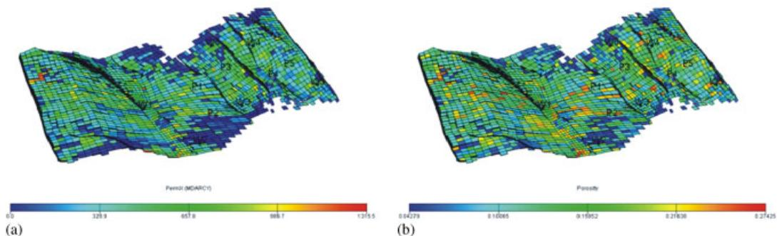
Figure 5. Permeability (a) and porosity map (b). Model three.
